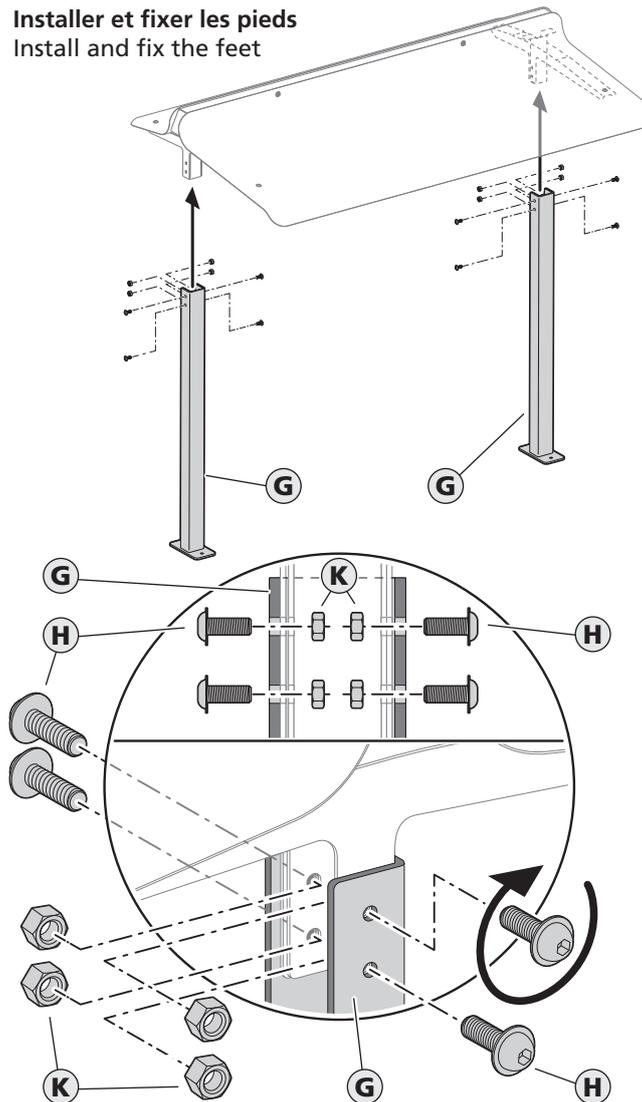
**FIXATION AU SOL / FLOOR FIXING**
